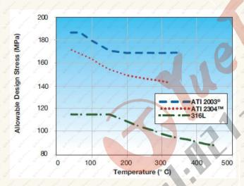
Maximum allowable design stress levels permitted for the use of ATI 2304<sup>™</sup>, ATI 2003<sup>®</sup>, and Type 316L plate under the ASME Boiler and Pressure Vessel Code Section VIII Division 1.
